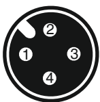
4-pin M12 built-in socket, A-coded
