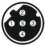
5-pin M12 built-in socket, D-coded
