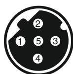
Prise encastrable M12 5 pôles, code D
