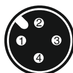
Prise encastrable M12 4 pôles, code A
