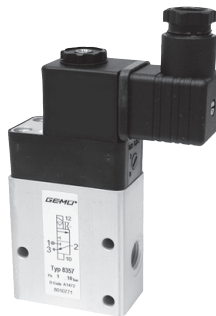
GEMÜ 8357 3/2-way metal pilot valve, servo assisted, aluminium DN 6 (15 - 150 psi)
