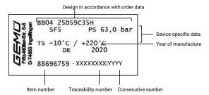
The month of manufacture is encoded in the traceability number and can be obtained from GEMÜ. The product was manufactured in Germany.
