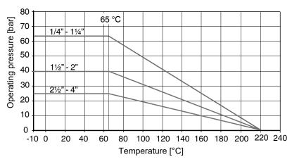
Use the clamped union with the correct pressure rating for a safe and correct pipeline design. Pressure ratings of the clamp alone are generally higher, but do not take into account the fully clamped assembly with gasket
