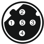
5-pin M12 built-in socket, D-coded
