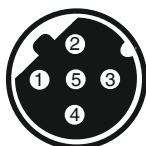
5-pin M12 built-in socket, D-coded
