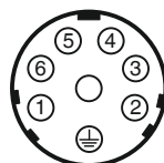
Plug assignment X2, S1/S2
