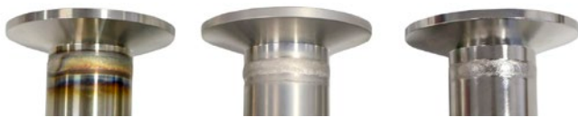
Figure 3: Untreated weld – pickled weld – pickled and electropolished weld
