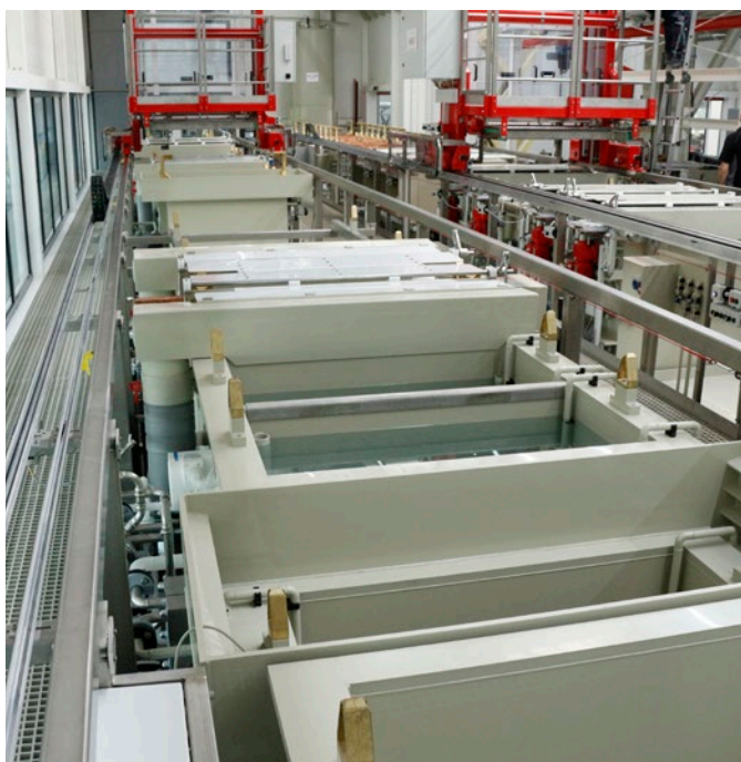
Figure 4: Fully automatic electropolishing system
