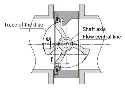
During operation, the disc directly disconnects from the seat, thereby reducing friction between the seat and disc, as well as the torque.
