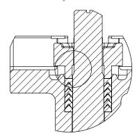
There is a chamfer at the upper end of the shaft which acts as an additional safety measure in case the shaft breaks.
