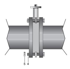
13. Slightly tighten the bolts 4 and nuts 5 diagonally.
