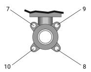
9. Tighten the nuts diagonally, counterhold with a wrench.
