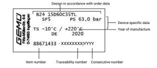
The month of manufacture is encoded in the traceability number and can be obtained from GEMÜ. The product was manufactured in Germany.
