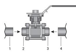
2. Align the pipes 1 and 4 on the left and right with the butt weld spigots 2 and 3, and attach them to the spigots.
