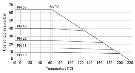
Pressure/temperature data in accordance with diagram refers to static operating conditions. Strongly fluctuating or fast-changing parameters can lead to a reduction of the service life. Special applications must be talked through with your technical contact person in advance.
