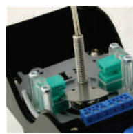
Fig. 8: Fixation of cam 1
