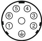
Plug assignment X2, S1/S2
