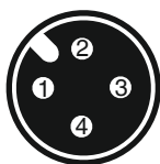
4-pin M12 built-in socket, A-coded
