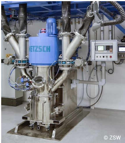
Production research at the ZSW: 60-litre mixing system for electrode pastes. Figure: ZSW
