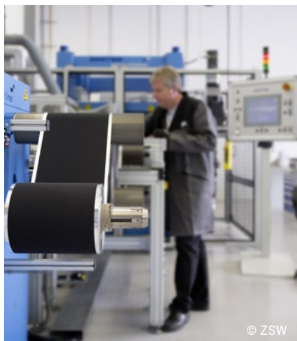
Production of electrode strips under near series conditions at the Centre for Solar Energy and Hydrogen Research (ZSW). Figure: ZSW
