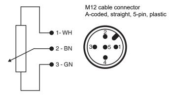
This design is suitable for connecting to the GEMÜ 1434, 1436 or 1435 positioner with the M12 cable connector design. For special versions X and Z:
