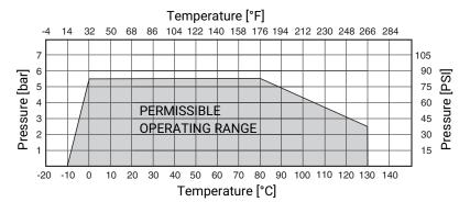
The pressure/temperature diagram is only an aid. The data refers to water as a working medium. A change of operating conditions or other media may result in deviations. In case of doubt it is advisable to test the behaviour of the material under the definited operating conditions by means of a test installation.
