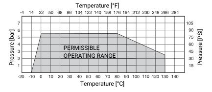
The pressure/temperature diagram is only an aid. The data refers to water as a working medium. A change of operating conditions or other media may result in deviations. In case of doubt it is advisable to test the behaviour of the material under the definited operating conditions by means of a test installation.
