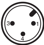
3-pin M12 plug, A-coded
