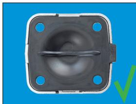
6. Then turn the diaphragm (with 2-piece diaphragms only the PTFE face) back anti-clockwise to the next possible bolt alignment (max. 180°). Ensure that the sealing weir and the diaphragm are aligned (return the PTFE face to its original shape).
