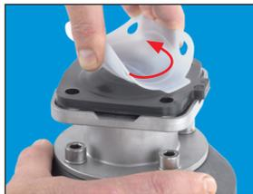
4. Unscrew the diaphragm from the spindle / compressor (Attention: right-hand thread, turn anti-clockwise to loosen it). Check the diaphragm for damage, if any.
