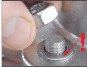
9. Insert the four bolts with their respective washers from the body side and tighten diagonally hand tight only. (Do not use force).
