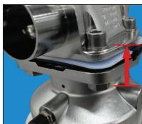
**15.** Move the pneumatic actuators to the closed position (move manual actuators only as far as the "half closed" position, open electrically-powered actuators approx. 20%).
