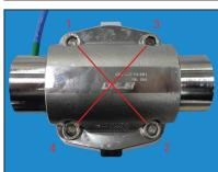
Loosen the connecting bolts diagonally and lift the actuator off the valve body.
