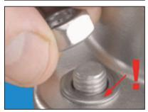
**14.** Insert the connecting bolts from the body side, position the nuts and bolt together diagonally so that they are hand tight (do not use force). Do not forget to use washers on both sides.
