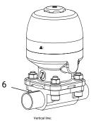
To mark the correct angle of rotation, line markings (6) are made on the valve body. The line markings enable simpler installation of the bodies in the system. The bodies have been positioned in a manner which is optimized for draining if the line markings point vertically upwards, as shown in the figure. The vertical line shall therefore form the reference line for the line markings.
