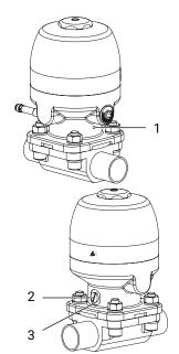
There is one bolt hole (1) with a minimum diameter of 2.4 mm in the distance piece of the actuator. This bolt hole serves as a leak detection hole if the diaphragm fails.
