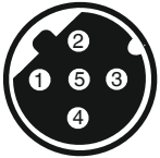
5-pin M12 built-in socket, D-coded
