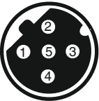
5-pin M12 built-in socket, D-coded
