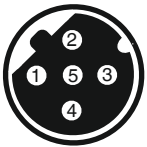
5-pin M12 built-in socket, D-coded
