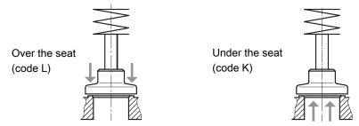
Under the seat (code K) is the preferred flow direction with incompressible liquid media to avoid water hammer The flow direction is indicated by an arrow on the valve body.
