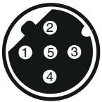
5-pin M12 built-in socket, D-coded
