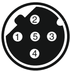
5-pin M12 built-in socket, D-coded
