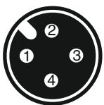
4-pin M12 built-in socket, A-coded
