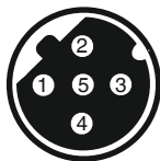
5-pin M12 built-in socket, D-coded
