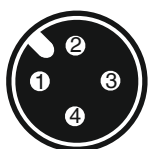
4-pin M12 built-in socket, A-coded
