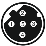
5-pin M12 built-in socket, D-coded
