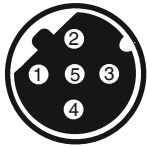
5-pin M12 built-in socket, D-coded
