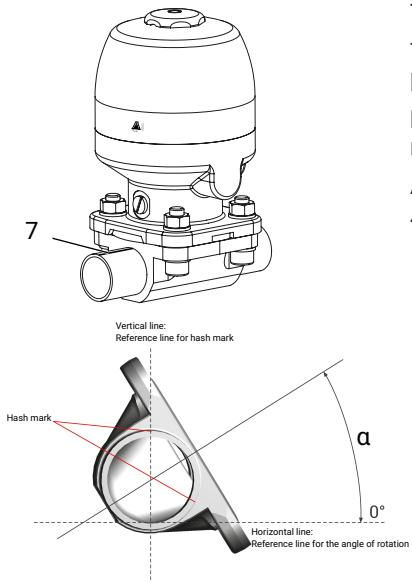
To mark the correct angle of rotation, line markings (7) are made on the valve body.
