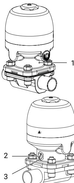
There is one bolt hole (1) with a minimum diameter of 2.4 mm in the distance piece of the actuator. This bolt hole serves as a leak detection hole if the diaphragm fails.
