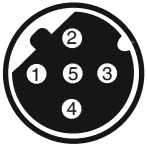
5-pin M12 built-in socket, D-coded
