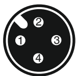
Prise encastrable M12 4 pôles, code A
